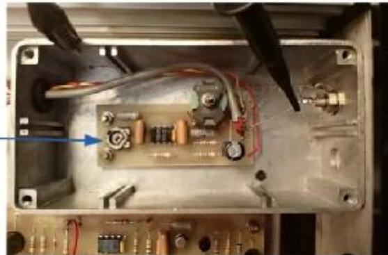
Connect ultrasonic transmitter to Kinelume and allow a warm up of 15mins to allow for stabilisation. Adjust the pot for an output frequency of 40kHz
