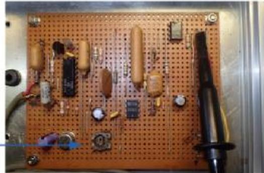
Allow a warm up of 15mins to allow for stabilisation. With the front panel sensitivity set at minimum, turn the pot anticlockwise until the voltage drops to -8V.
