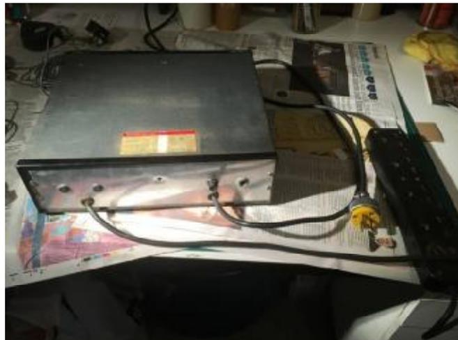
Immediately the mains wiring gave cause for concern and when powered up, occasionally the office RCB tripped indicating earth leakage issues. This was hardly surprising given that that mains suppression inductors were burnt out.
