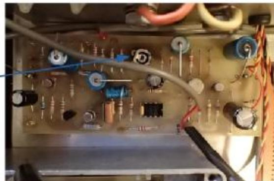
Allow a warm up of 15mins to allow for stabilisation. Turn the pot fully clockwise. With the ultrasonic receiver disconnected turn the pot anticlockwise until the voltage suddenly drops
