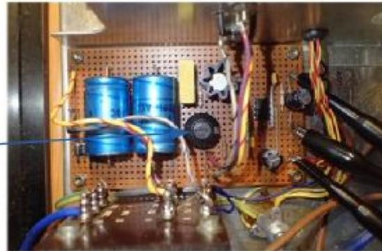
Allow a 15min warm-up period. adjust VR1 for an output voltage of  $\pm 10\text{Vdc}$
